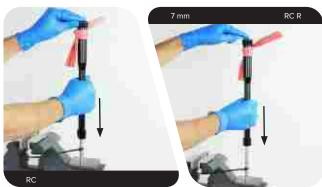
Install the Charger Damper RC or RC R assembly into the damper side upper tube. Thread the top cap into the upper tube and tighten it
