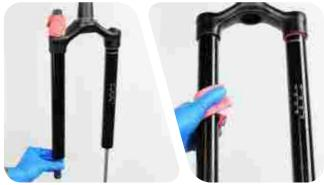
Remove the compression damper top cap o-ring and piston u-cup seal. Apply grease to the new o-ring and seal, and install them.
