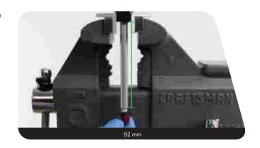
Pour 3wt suspension oil into the tube until the oil is just below the purge holes.
