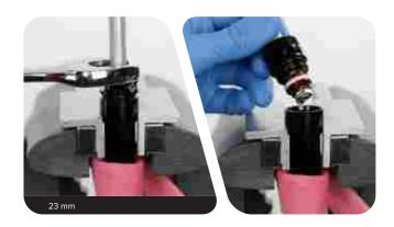
Remove the seal head from the rebound damper shaft and discard it.
