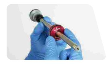
Apply red Loctite 2760 to the first two to three full threads on the end of the air shaft.
