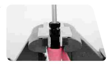
Unthread and slowly remove the rebound damper seal head assembly from the cartridge tube.
