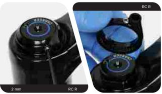
RCT R: Remove the low speed knob/remote spool assembly.
