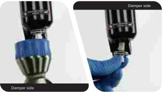
Firmly pull the lower leg downward until fluid begins to drain. Continue pulling downward to remove the lower leg.
