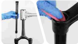
Clamp the cartridge tube into a vise with Charger RC/RL Vise Blocks.
