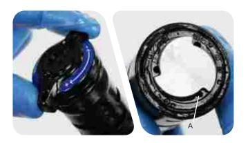
Insert the compression damper into the upper tube. Press down slowly and rotate in a circular motion until the damper is installed.
