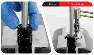
Thread the rebound bottom bolt into the shaft 3-4 turns.
