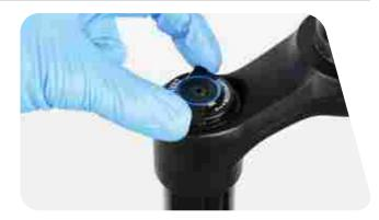
Remove the retaining screw and remove the knob (RC) or remote spool (RC R).
