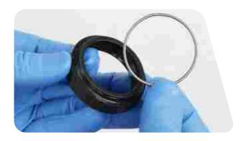
6 Insert the narrow end of a new wiper seal into the recessed end of the 35 mm Dust Seal Installation tool.
