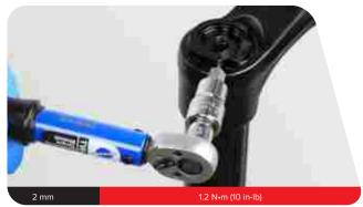
Install the remote spool onto the hex adjuster with the cable set screw oriented in the 10 o'clock position, =30 degrees from center.
