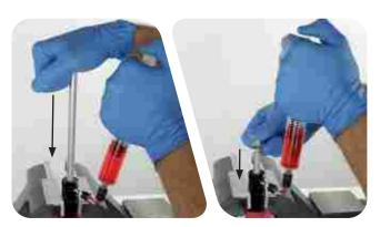
Pull the rebound damper shaft slowly out of the cartridge tube while applying opposing pressure on the syringe plunger as oil fills the damper.
