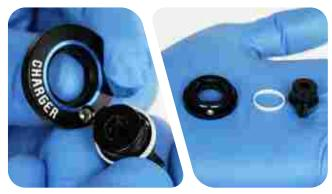
Install the remote spool onto the hex adjuster with the spool cable set screw oriented within the  $87^{\circ}$  range zone.
