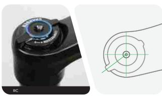
Install and tighten the retaining screw.
