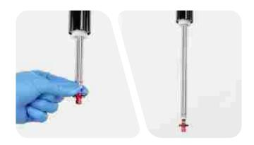
Remove the rebound damper and seal head.
