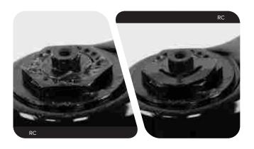
**60** RC: Install the adjuster knob with the tab in the 7-8 o'clock, unlocked, position.
