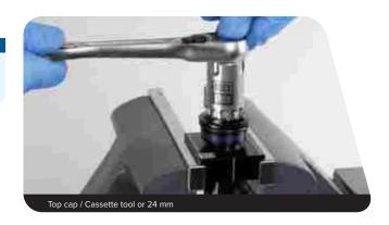
Carefully remove the compression damper.
