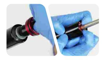
9 Retaining rings have a sharper-edged side and a rounder edged side. Installing retaining rings with the sharper-edged side facing the tool will allow for easier installation and removal.
