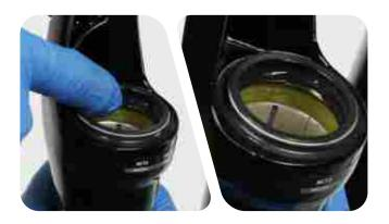
Install the lower leg assembly onto the upper tubes and slide it just enough to engage the upper bushings with the upper tubes.
