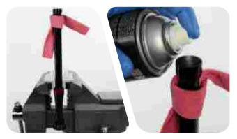
Squeeze the bladder 5-6 times to circulate the cleaner into the damper.
