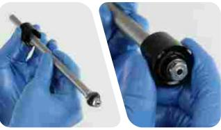
Insert the rebound adjuster knob into the rebound damper and rotate it counter clockwise until it stops. This is the full open position.
