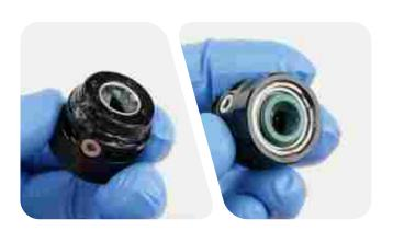
Install the new seal head onto the rebound damper shaft, threaded end first, and slide it towards the piston until it stops.
