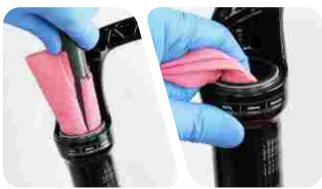
Install the foam rings under the wiper seals.
