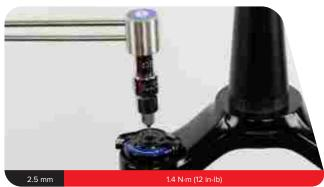
6b RC R: Install the cable stop collar with the housing guide in the 6 o'clock forward position, oriented outward ≈20°-30° degrees from center.
