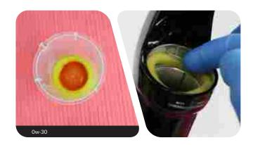
Remove the outer wire spring from each new dust wiper seal and set them aside.
