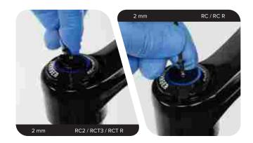
RC2 / RCT3 / RC: Remove the low speed compression adjuster knob.
