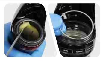
Stabilize the lower leg on a bench top. Place the tip of a downhill tire lever under the wiper seal. Press down on the downhill tire lever handle to remove the seal.
