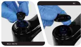
RC2 / RCT3: Remove the compression mode adjuster knob.
