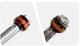
Apply grease to the new rebound damper seal head seals.
