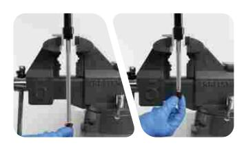
Push the rebound damper into the cartridge tube until there is **92 mm** (length) of shaft extended. Do not push the damper into the tube any further.
