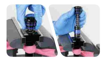
Remove the cartridge tube and rebound damper assembly from the vise and pour the oil into an oil pan.
