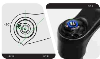
Install and tighten the remote spool retaining screw.
