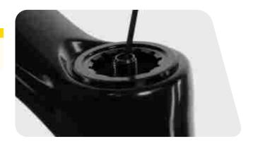
Turn the rebound adjuster knob counter-clockwise until it stops. This is the full open/fast rebound setting.
