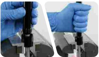
Secure a shop towel around the cartridge tube to absorb oil.
