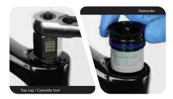
Remove the top cap o-ring and discard it. Apply grease to a new o-ring and install it.
