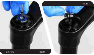
RC R: Loosen the set screw and remove the cable stop clamp.
