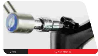
Install the lower remote spool (A) onto the hex adjuster. Install the upper spool with the alignment indicator dot (B) positioned within the range bracket (C).
