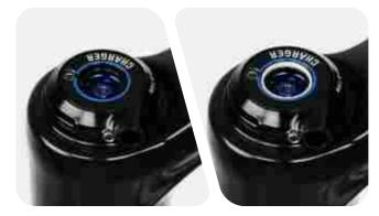
Install the low speed adjuster knob onto the hex adjuster. Install and tighten the knob retaining screw.
