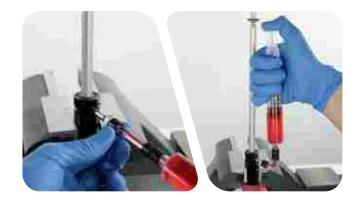
Push the rebound damper shaft into the cartridge tube while applying opposing pressure on the syringe plunger as the syringe fills with oil.
