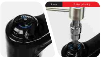
**RC R:** Install the cable stop collar with the housing guide in the 6 o'clock forward position, oriented outward ≈20° degrees from center.
