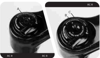
Install the spool retaining screw, thread it in and stop when it contacts the upper spool. Do not tighten the screw.
