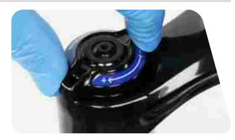
2 Remove the retaining screw and remove the knob (RC) or remote spool (RC R).
