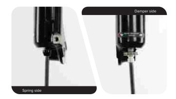
5 Strike each bottom bolt to dislodge the shafts from the lower leg on each side. The bolt head should contact the bottom of the lower leg.
