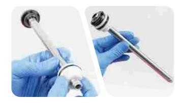
Insert the rebound damper and seal head into the upper tube.
