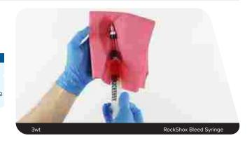
Thread the syringe bleed fitting into the seal head bleed port.
