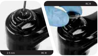
RC: Remove the detent spring.
