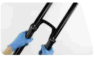
The inside bottom of the lower leg should not contact the spring or damper shafts. A gap between the shaft ends and the lower leg bolt holes should be visible.
