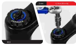
**RC:** Install the compression adjuster knob onto the top cap with the tab in the forward, unlocked, position.
