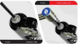
Install the rebound damper knob and tighten the set screw.
