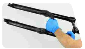
The spring and damper shafts should be visible through the bottom bolt holes.
