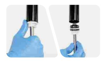
Clean the inside and outside of the upper tube. Inspect the inside and outside of the upper tube for scratches.
