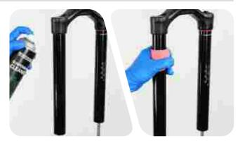
Apply grease to the inner surfaces of the dust wiper seals.
