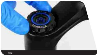
RC2 / RCT 3: Install the low speed compression adjuster knob onto the hex adjuster rod
