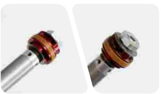
Apply grease to the inner seal and bushing in the new rebound damper seal head.  $\,$
