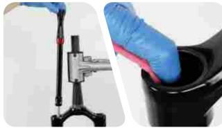
Remove the o-ring from the top cap. Clean the top cap threads and o-ring groove. Apply grease to a new o-ring and install it.
