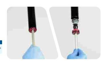
Clamp an 8 mm hex wrench into a vise. Position the air piston onto the hex wrench. While holding the air shaft, unthread and remove the air shaft nut from the air spring shaft.
