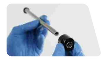
Spray RockShox Suspension Cleaner or isopropyl alcohol into the cartridge tube and clean the inside of the tube with a clean shop towel and a thin dowel (≤16 mm diameter).
