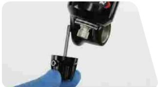
Place an oil pan beneath the fork to catch the draining oil.
