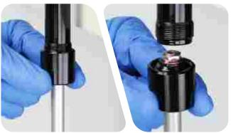
Remove the seal head from the rebound damper shaft.
