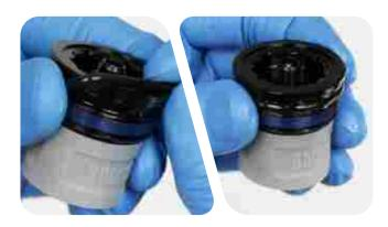
Push the air shaft into the upper tube with your thumb. While holding the shaft in, remove the retaining ring. Slide the retaining ring onto your thumb and carefully release the air spring shaft.
