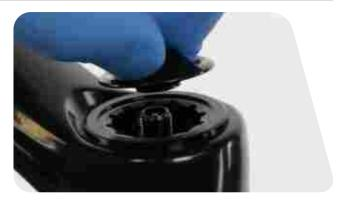
Depress the Schrader valve and release all air pressure.
