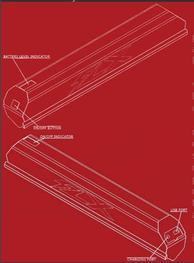
Removing the battery from the bike when storing it for a long period of time is recommended. In this case store it in a cool, dry area away from water. The charge left in the battery should be 50%-75% for long storage times.
