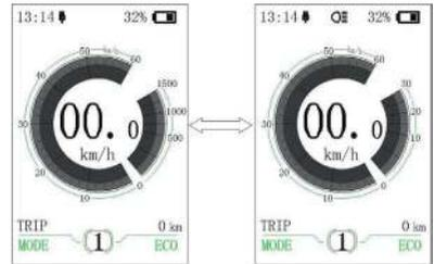
(6) "SOC View" --- set display mode for battery level
