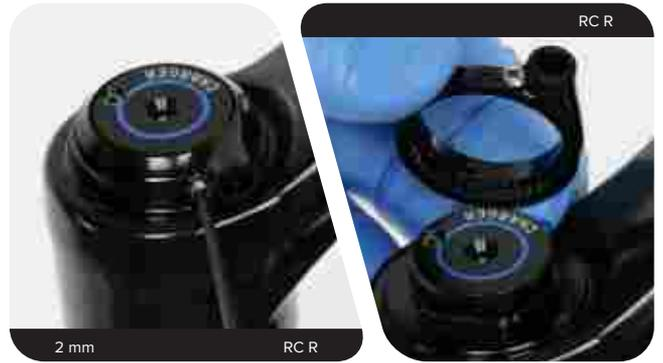
**5** **RCT R:** Remove the low speed knob/remote spool assembly.
