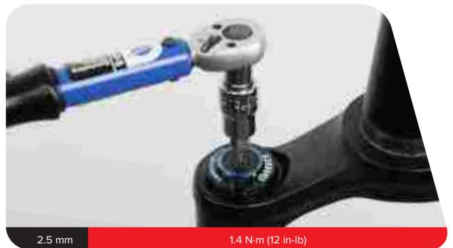
**3 RC R:** Install the cable stop collar with the housing guide in the 6 o'clock forward position, oriented outward  $\approx 50^\circ$  degrees from center.
