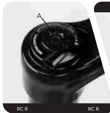
Install the spool retaining screw, thread it in and stop when it contacts the upper spool. Do not tighten the screw.
