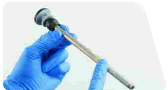
**4** Apply grease to the new seal head inner seal.
