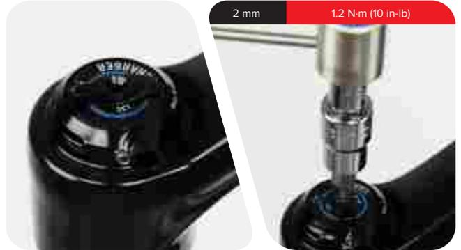
**RC R:** Install the cable stop collar with the housing guide in the 6 o'clock forward position, oriented outward  $\approx 20^\circ$  degrees from center.
