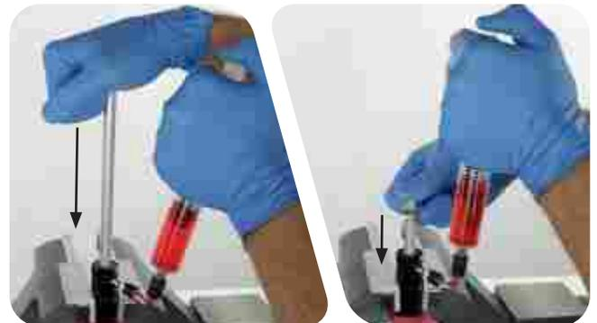
Pull the rebound damper shaft slowly out of the cartridge tube while applying opposing pressure on the syringe plunger as oil fills the damper.
