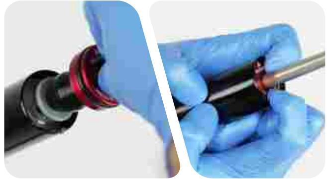
**9** Retaining rings have a sharper-edged side and a rounder edged side. Installing retaining rings with the sharper-edged side facing the tool will allow for easier installation and removal.
