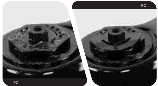
**6a** **RC:** Install the adjuster knob with the tab in the 7-8 o'clock, unlocked, position.
