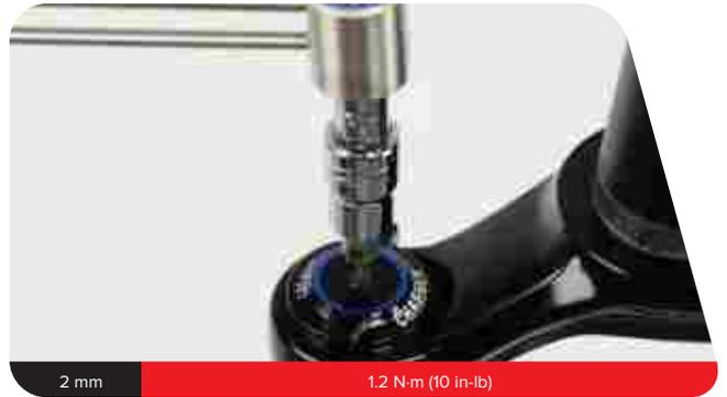
**3b RCT R:** Install the cable stop collar with the housing guide in the 6 o'clock forward position, oriented outward  $\approx 20$  degrees from center.
