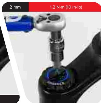
**RC:** Install the compression adjuster knob onto the top cap with the tab in the forward, unlocked, position.
