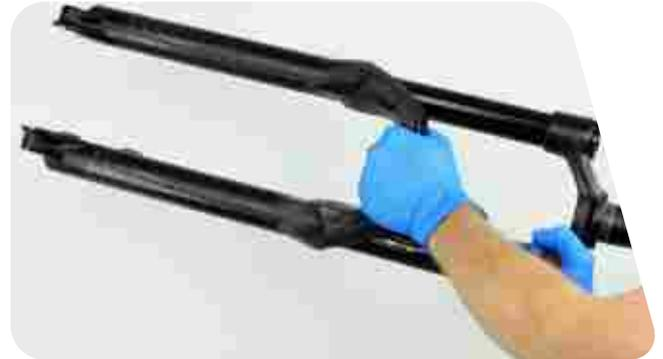
The spring and damper shafts should be visible through the bottom bolt holes.
