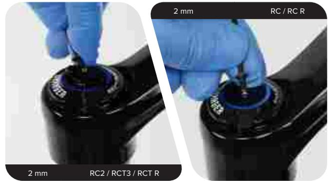
**3** **RC2 / RCT3 / RC:** Remove the low speed compression adjuster knob.
