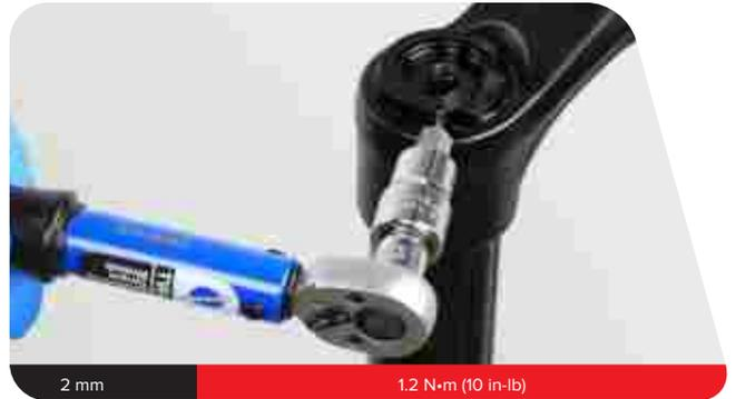
Install the remote spool onto the hex adjuster with the cable set screw oriented in the 10 o'clock position,  $\approx 30$  degrees from center.
