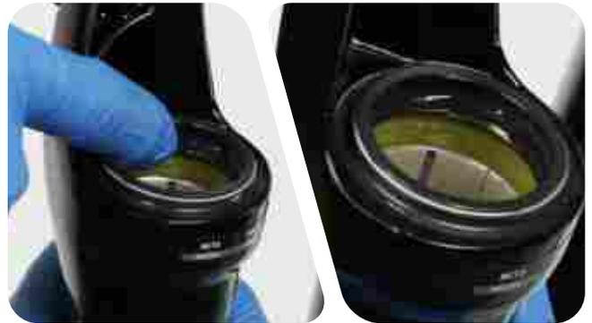
**3** Install the lower leg assembly onto the upper tubes and slide it just enough to engage the upper bushings with the upper tubes.
