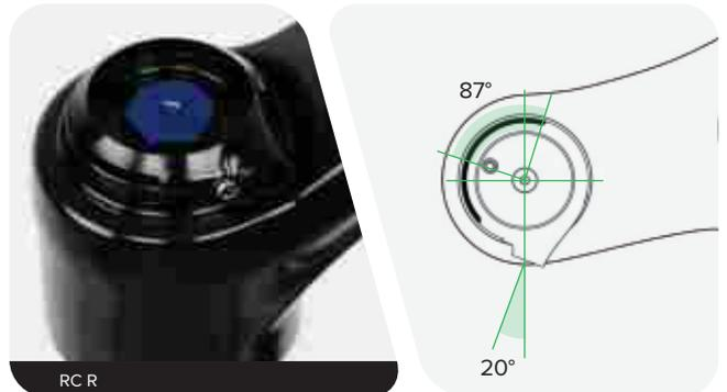
Install the remote spool onto the hex adjuster with the spool cable set screw oriented within the 87° range zone.
