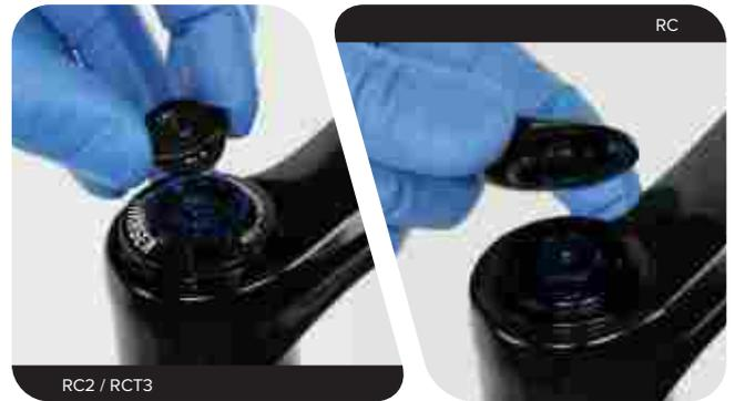
**RC2 / RCT3:** Remove the compression mode adjuster knob.
