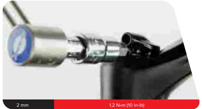
Install the lower remote spool (A) onto the hex adjuster. Install the upper spool with the alignment indicator dot (B) positioned within the range bracket (C).
