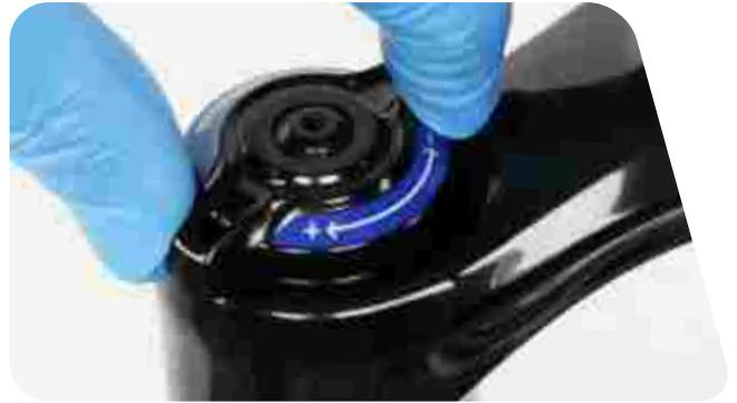
**2** Remove the retaining screw and remove the knob (RC) or remote spool (RC R).
