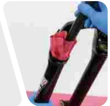
Replace the o-ring or seal with a new one from the service kit. Use your fingers or a pick to pierce and remove the old seal or o-ring.
