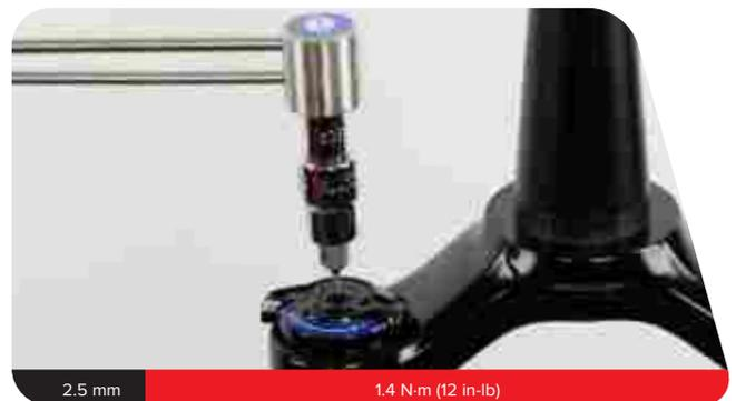
**6b RC R:** Install the cable stop collar with the housing guide in the 6 o'clock forward position, oriented outward  $\approx 20^{\circ}$ - $30^{\circ}$  degrees from center.
