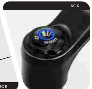
Install and tighten the remote spool retaining screw.
