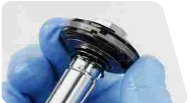
**5** Install the seal head onto the rebound damper shaft.
