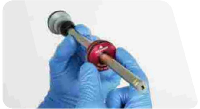
**6** Apply red Loctite 2760 to the first two to three full threads on the end of the air shaft.
