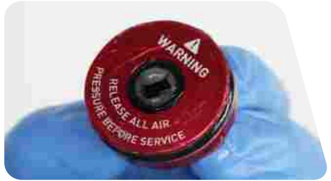
**5** Install the new seal head assembly onto the air shaft.
