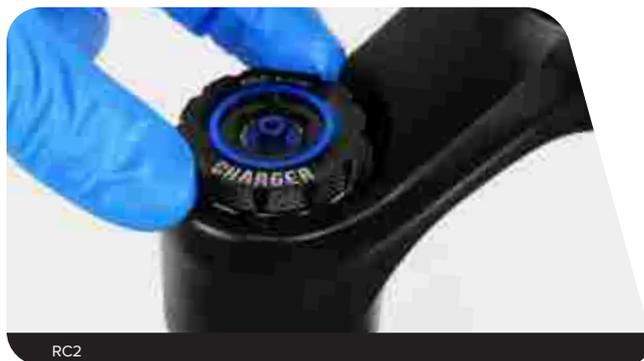
**RC2 / RCT 3:** Install the low speed compression adjuster knob onto the hex adjuster rod. Install and tighten the retaining screw.
