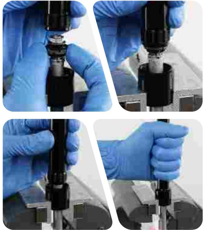
**4** Secure a shop towel around the cartridge tube to absorb oil.
