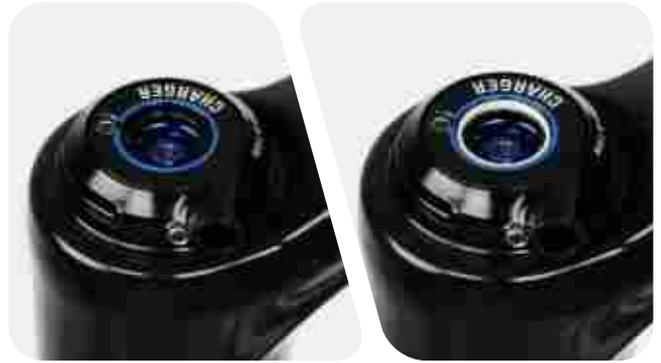
Install the low speed adjuster knob onto the hex adjuster. Install and tighten the knob retaining screw.
