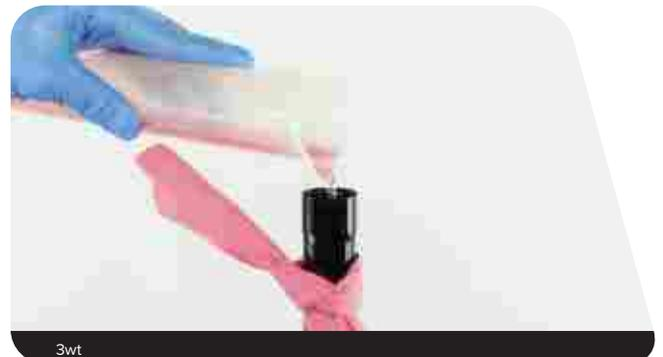
**5** Thread a bottom bolt into the rebound damper shaft.
