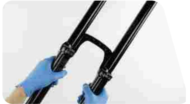
The inside bottom of the lower leg should not contact the spring or damper shafts. A gap between the shaft ends and the lower leg bolt holes should be visible.
