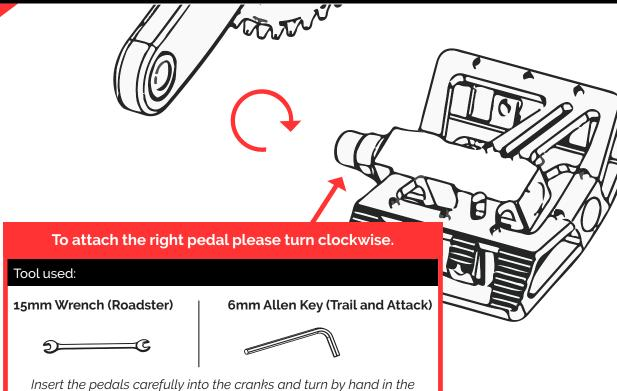
direction shown. Tighten with the appropriate tool provided.
